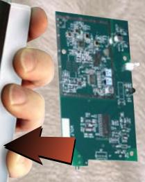
Berkeley's custom, calibrated receiver demodulates and displays both PCS and Cellular frequency bands in true dBm
